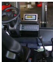
KPZ 39 Hydraulic Forklift scale
