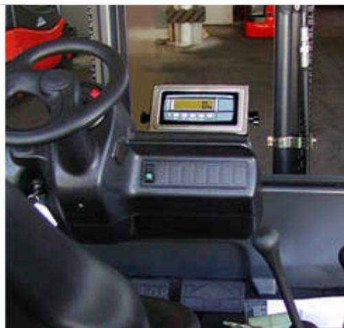
Every fork truck can in principle be equipped with the weight indicator KPZ 39-1, an additional do it your selv assembling at every fork truck is easily possible. The weight indicator KPZ 39- 1 has extra been developed for the rugged fork truck operation in the hardest industry input.
