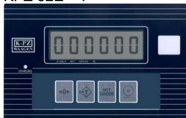
**Features:** High resolution and fast weight display. Built in a stable, robust steel housing, user-friendly, dust and waterproof membrane keyboard, 4 large control buttons. LCD - display, 6 digits, 1.18"/30mm high digits, backlit. For approved weighing applications.
