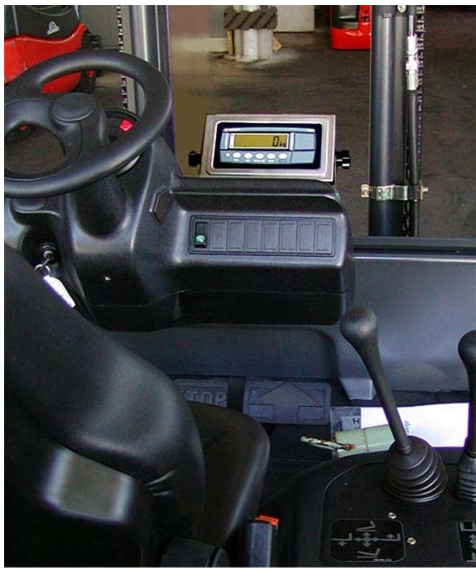
**Transport and weighing in one operation !!!**
