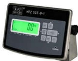
**Description:** solid stainless steel housing IP 67, user-friendly, large function keys. LCD display: 6 digit, various symbols, backlight. Operating temperature from -10°C up to +40°C.
