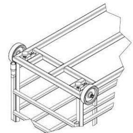
KPZ 2A, low profile Animal platform scale, dim 920 x 2200 mm, robust and stable, high quality steel construction with structured plate, Galvanized version with a galvanized raw framework, Load cells : 4 high quality, OIML approved C 3, DMS load cell, IP 68, type KPZ 502E-3. Weighing Indicator : KPZ 52E91 – sensitive Animal Filter
