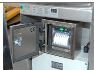
Build in Thermo Printer IP65 housing
